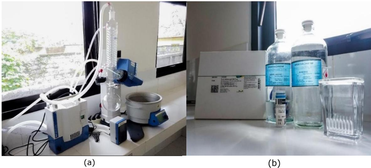
Gambar 6. *Rotary evaporator set (a) dan bahan kimia (b).*
